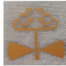
Figure 1: A 2 \times 2 60 GHz antenna array on glass substrate with CPW to MS transition feeding element.
